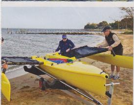
frames) slot into reinforced holes in the main hull, and simple tensioning lines lock them in (as does the rig when the shrouds are attached). Once they stepped the 9-pound carbon rig, lashed the screecher to the carbon sprit, raised the sails (with external halyards), dropped in the carbon kick-up rudder, and ran the sheets, they were off and blazing. An International 14-type tinkerer's boat this is not; it's a sail-it-out-of-the-box, one-design gem.
