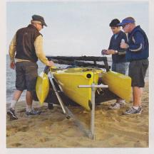
BOTY judge Chuck Allen three-sailed the Weta Trimaran with ease in 20 knots. From trailer to water is a quick affair: drop the lightweight floats (with carbon beams) into the main hull, step the rig, hoist the sails, and go sailing.
